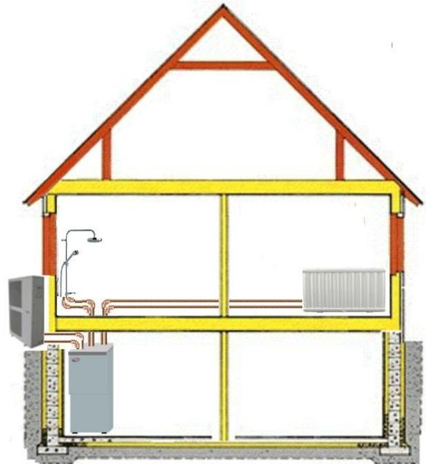
During heating of the house the 3-way valve and the main circulating pump drives water to flow from the heat pump through the radiator system of the house. If extra power is needed, the electric heater will be turned on to assist the heat pump.
